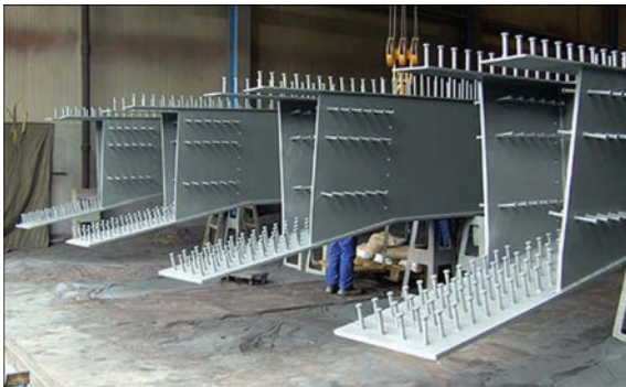
Fig. 13. Shear studs in civil engineering (source: Schöler + Bolte)
