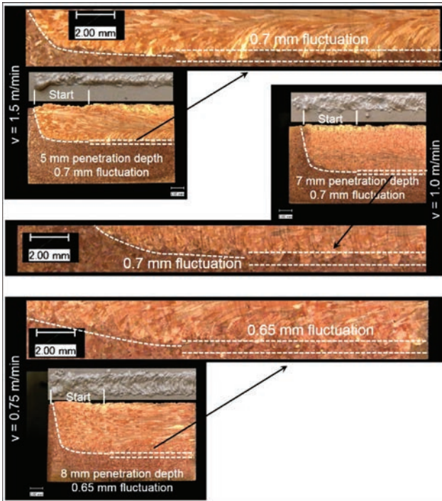
Fig. 4. LaVa-welding of copper — penetration depth and fluctuation of penetration at different welding velocities
