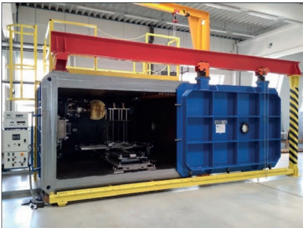
Fig. 1. PZ EZ 30 STU electron beam welding machine
