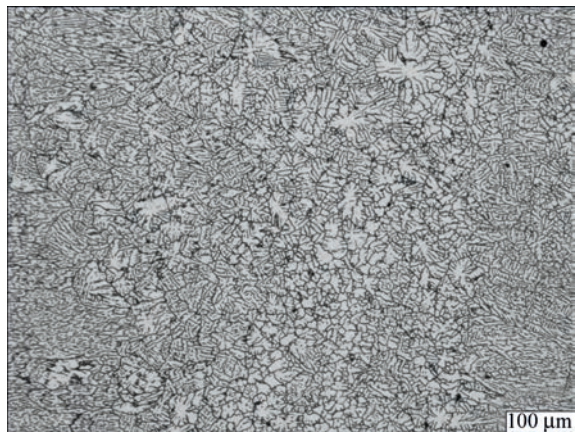
Fig. 5. The microstructure of the equiaxed dendrite zone in the weld metal centre ( I_B = 60 \text{ mA} , v = 50 \text{ mm/s} )
