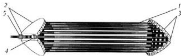
Figure 2. Optical scheme of the GIBRID laser head for single beam generation: 1 – 20 discharge tubes; 2, 3 – deflecting mirrors; 4 – non-transmitting mirror; 5 – output mirror
