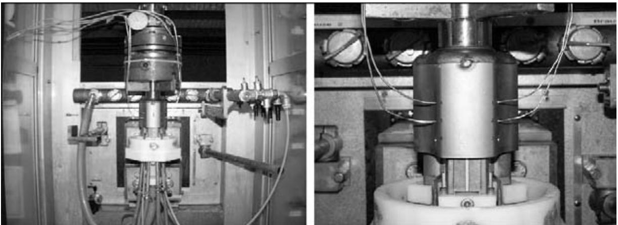
**Figure 5.** Experimental arrangement for temperature measurement during induction hardening
