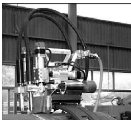
Figure 3. Automatic welding carriage developed
