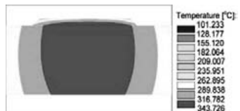
Figure 24. Numerically calculated temperature distribution in layer 1 after 120 s of cooling phase
