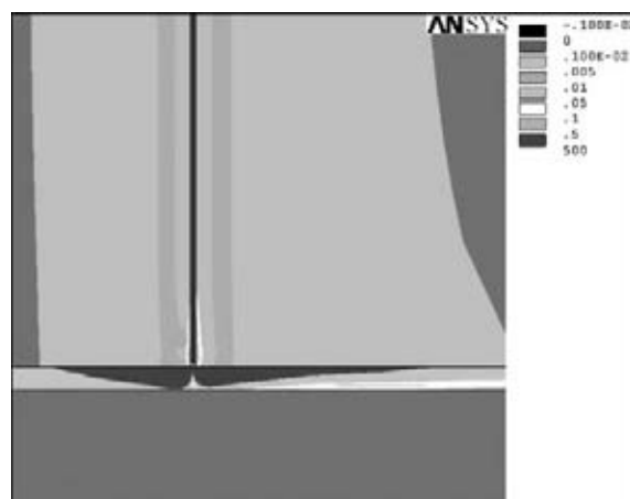
Figure 6. Contour of magnetic flux density at current of 400 A
