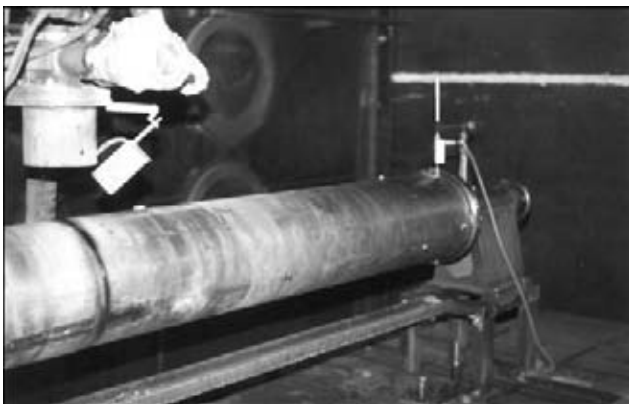
Figure 4. Thermal straightening of the VT-1 titanium alloy shell 6 m length, 350 mm diameter and 6 mm wall thickness having longitudinal axis bend distortions
