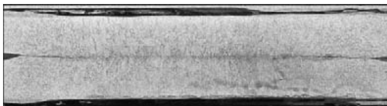
Figure 10. Macrostructure of spot welded joint with small weld nugget of about 2.0 mm in diameter: I = 7.3 kA, t = 20 pulses, P = 190 daN ( \times 40 )
