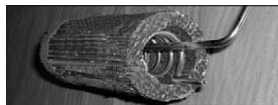
Figure 10. Spiral structure pushed inside SiC tube
