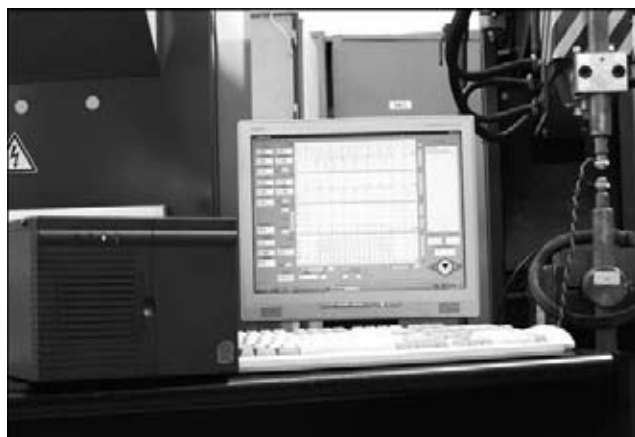
Figure 2. LOGWELD measuring and recording device
