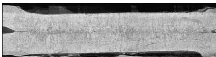
Figure 9. Macrostructure of spot welded joint with correctly formed nugget of diameter close to electrode lap diameter ( d_j = d_e = 5\sqrt{\delta} ): I = 8.3 kA, t = 20 pulses, P = 190 daN ( \times 40 )
