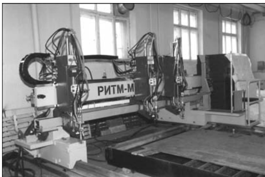
Figure 1. RITM-M gas cutting machine with 1-4 torches
