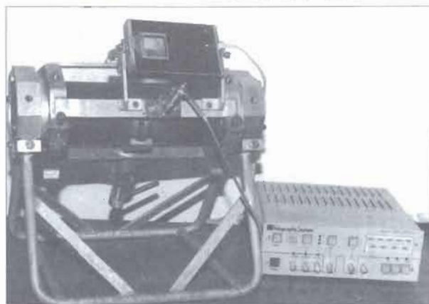
Figure 2. General view of a holographic unit for nondestructive quality control of elements of tubular structures
