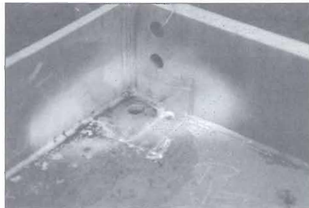
Figure 2. Zinc drain opening and crack propagating from the web plate to the cross-piece through the fillet weld
