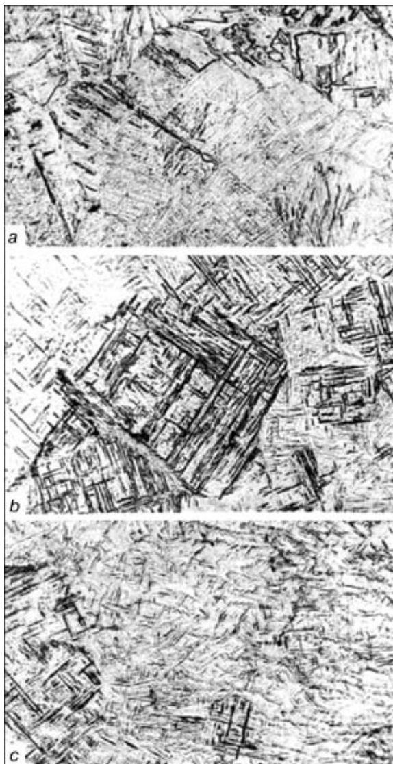
Figure 3. Microstructure of the HAZ metal in the joints made by arc (a), electron beam (b) and laser welding (c) ( \times 400 ) (reduced by 4/5)
