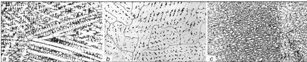
Figure 4. Microstructures of A-TIG weld metal on different nickel alloys: a – Nimonic-75; b – Inconel 600; c – Hastelloy X
