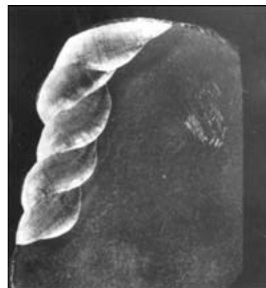
Figure 1. Macrosection of a built-up rail lip
