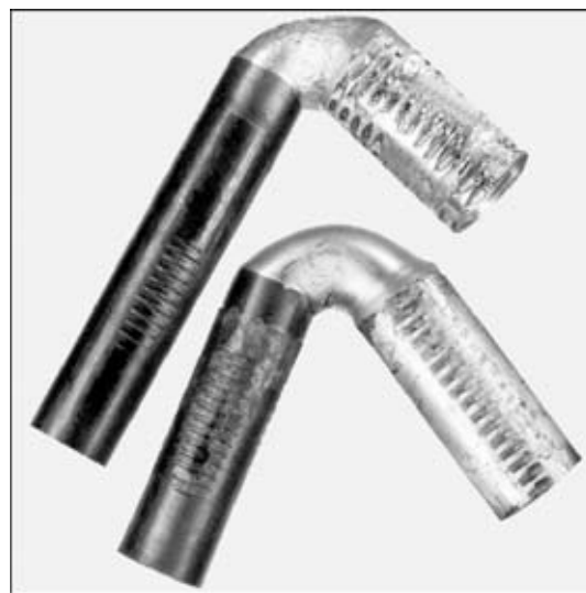
Figure 6. Welded joints ( P_h = 40\text{--}60 MPa, P_f = 200 MPa, t_h = 0.4 s, t_b = 0.7 s) after impact bending tests
