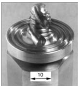
Figure 13. Prototype of a tool with MX Triflute trade mark
