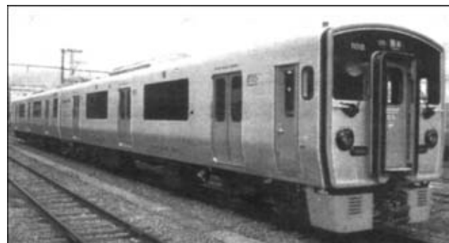
Figure 25. Railway car, made by Hitachi, using FSW
