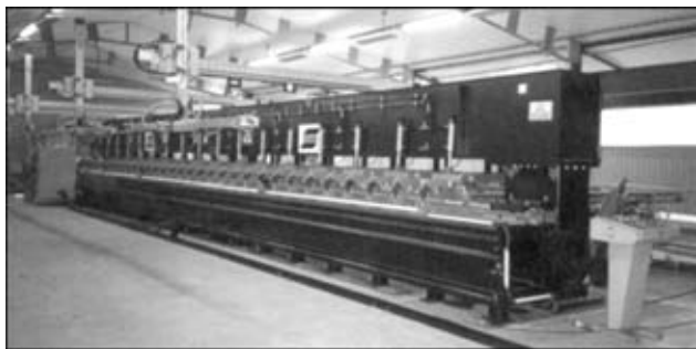
Figure 20. ESAB Super Stir™ machine for welding extruded panels, supplied to Marine Aluminium, Norway
