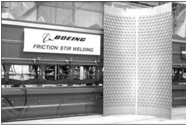
Figure 22. Fragment of a fuel tank of «Delta» missile with FSW longitudinal weld
