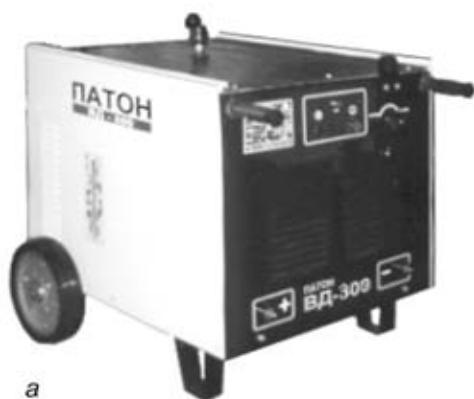
Figure 2. Appearance of rectifier VD-309 (a), volt-ampere characteristic of auxiliary (1) and operating (2) rectifier (b)
