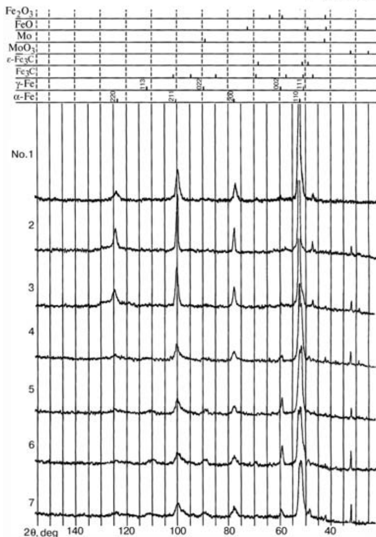
Figure 3. X-ray patterns of surfaces of an initial sample and samples after PDT (treatment parameters are given in Table 2)
