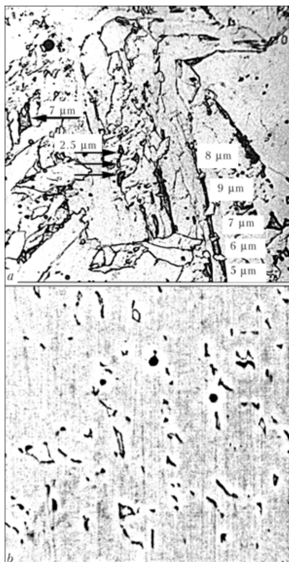
Figure 5. Microstructure of low-alloy (a) and with ULCC (b) weld metal with MAC-phase ( \times 1000 )
