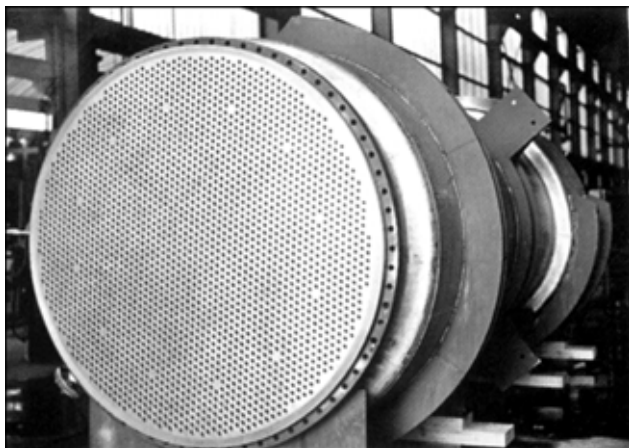
Figure 4. Heat exchangers made using a bimetal (steel + titanium) tubesheet
