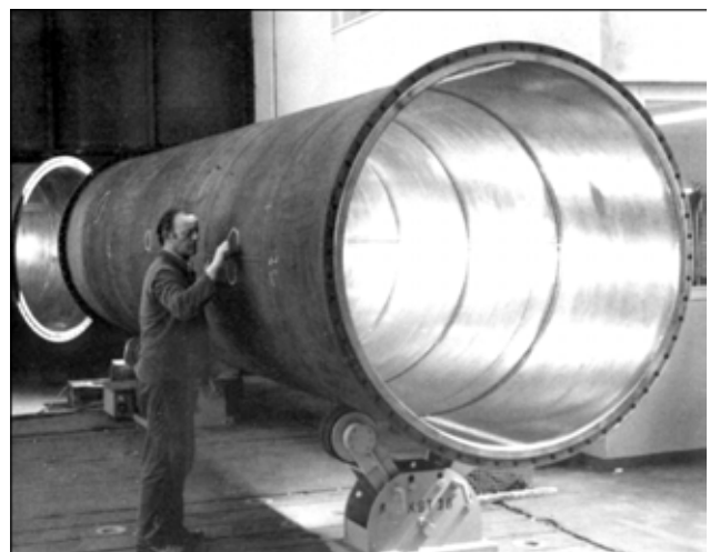
Figure 3. Pipe of 1500 mm diameter clad on the inside by a tantalum layer using EW
