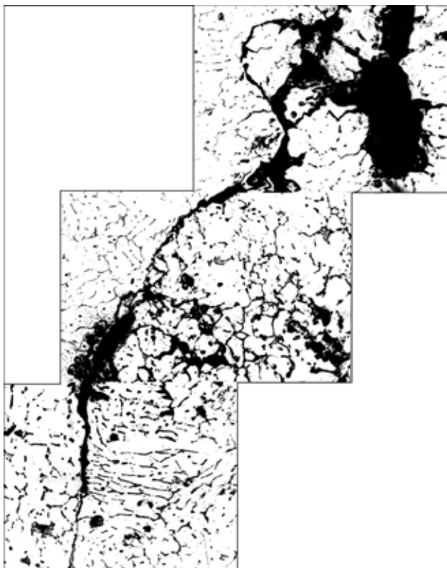
Figure 10. Microstructure of AMts alloy ingot with oxide films and discontinuities (distance from the ingot surface is about 10 mm) ( \times 200 )
