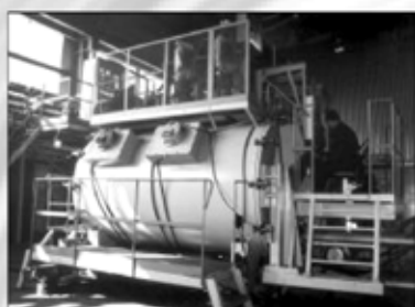
Appearance of electron beam unit UE 185 for ingot surface melting
