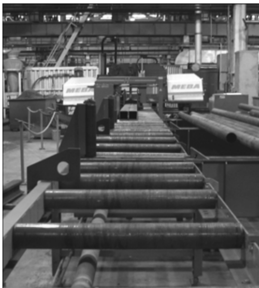
Figure 4. CNC cutting line on the basis of bi-column band saw MEBA 560 GA-3300
