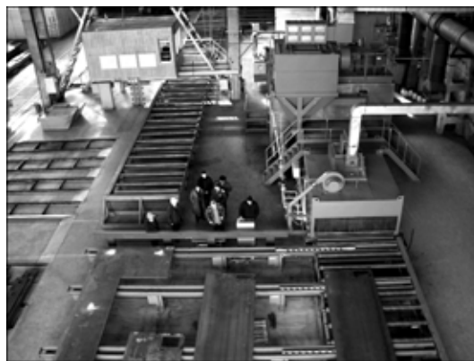
Figure 5. The Guttman shot-blast cleaning and priming line
