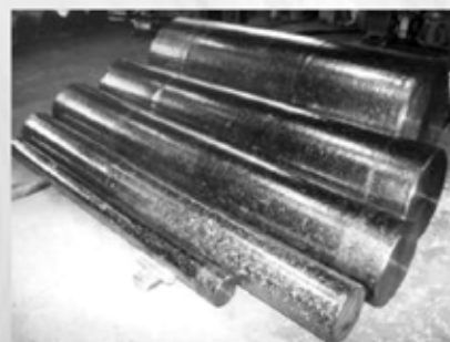
Titanium ingots of 110-600 mm diameter after surface melting
