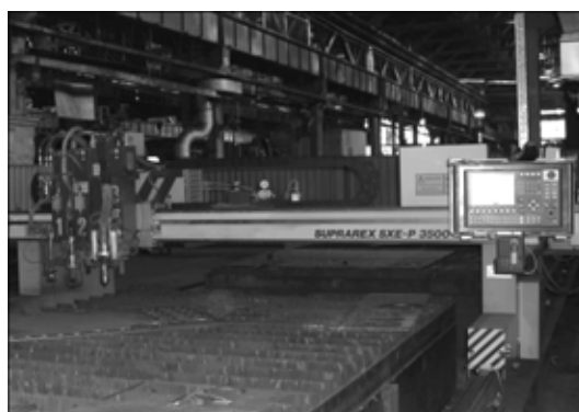
Figure 3. Machine for thermal cutting Suprarex SXE-3500 with CNC
