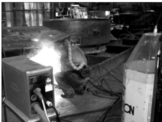
Figure 1. Welding of metal structure using the Fronius semi-automatic machine of «new generation» with cassette of increased capacity of Marathon type (mass of welding wire is 475 kg)
