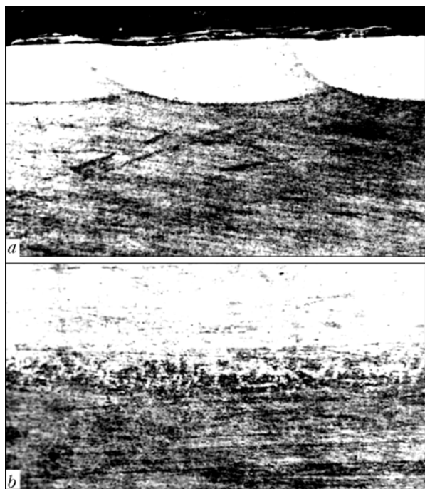
Figure 5. Microstructure of the chromium layer deposited by the combined method on steel 38KhN3MFA (the process was carried out with overlapping of strips at K_0 = 24\% ): a — strip structure ( \times 50 ); b — transition zone ( \times 500 )
