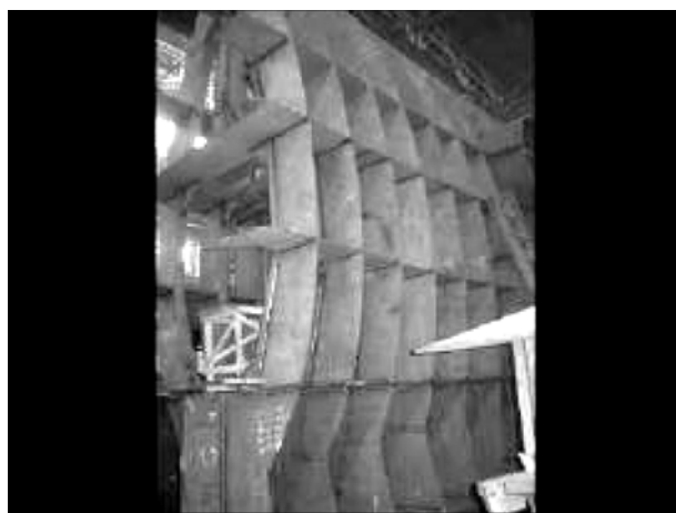
Figure 6. Fragment welded with rutile flux-cored wire (ASME 5.20 E71-T1)
