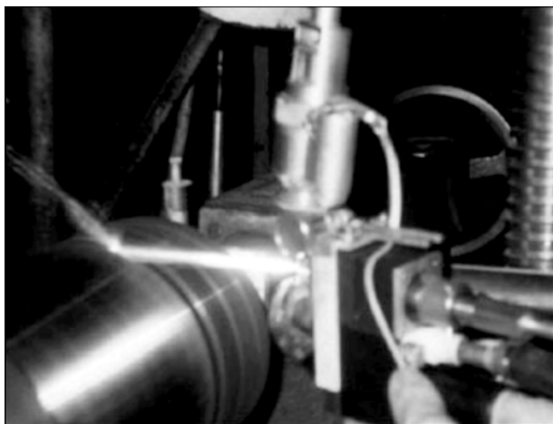
Figure 1. Laser-microplasma coating and alloying of cylindrical parts
