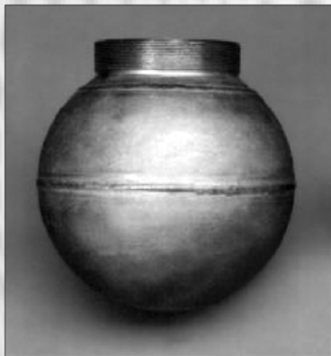
Typical example of TIG-F welding
