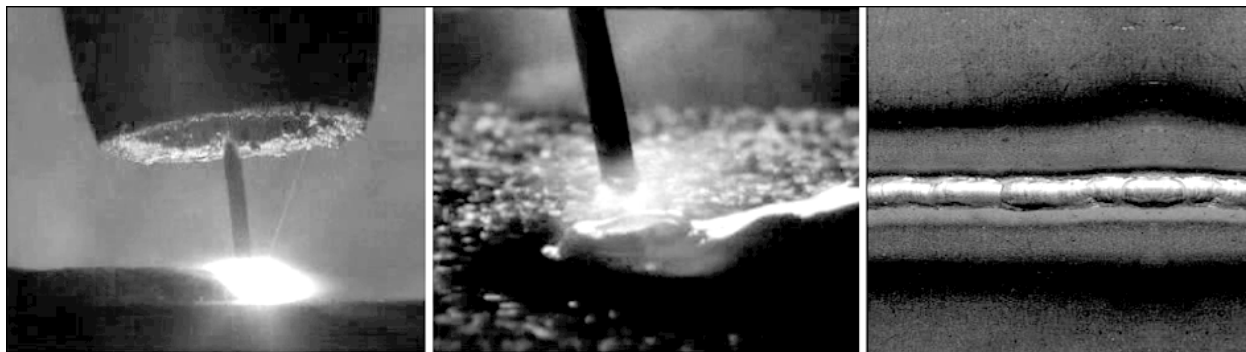
Figure 1. Dynamic scenes of «Navigator» showing formation of weld pool and weld
