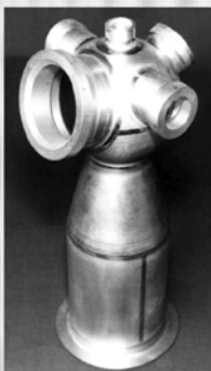
Stamped-welded body of rocket engine made from molybdenum
