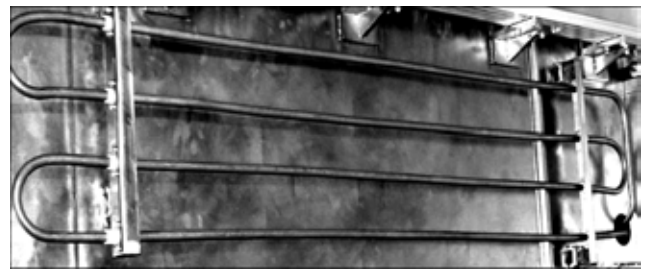
Figure 1. General view of cryocoil mounted on rear wall of vacuum chamber of KL-132 installation (below to the right is «cold inlet» into vacuum chamber)
