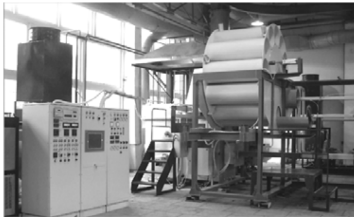
Experimental-industrial unit for steam-plasma processing of environmentally hazardous wastes
