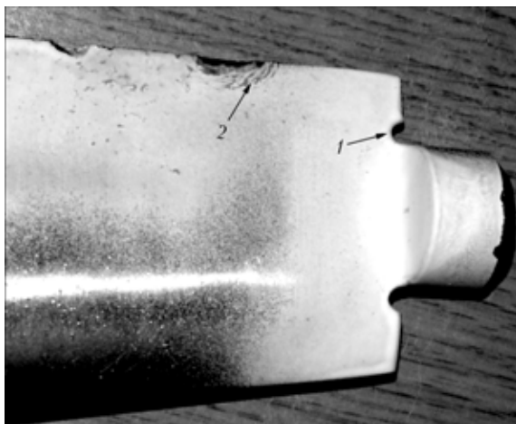
Figure 1. Fatigue-corrosion fracture (1) of the surface of 14Kh17N2 steel blade formed during operation, and brittle fracture within the nick regions (2) formed in emergency fracture
