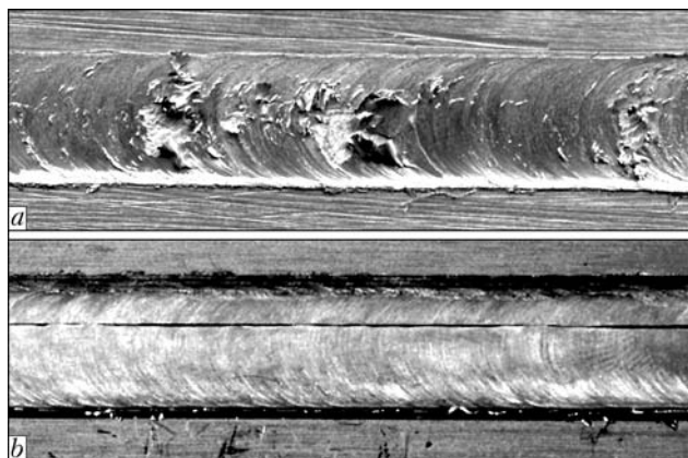
Figure 3. Appearance of the face surface of welds produced by FSW of aluminium alloy 1420 2 mm thick at excess ( a ) and insufficient ( b ) immersion of the lip into the metal being welded ( \times 2 )
