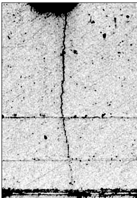
Figure 4. Microstructure of 17G1S steel specimen with corrosion crack
