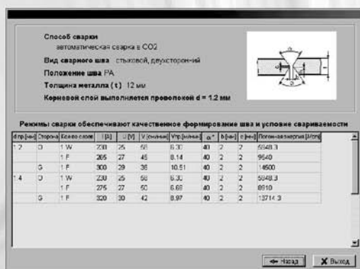
Figure 2. Information on CO 2 welding of butt joint
