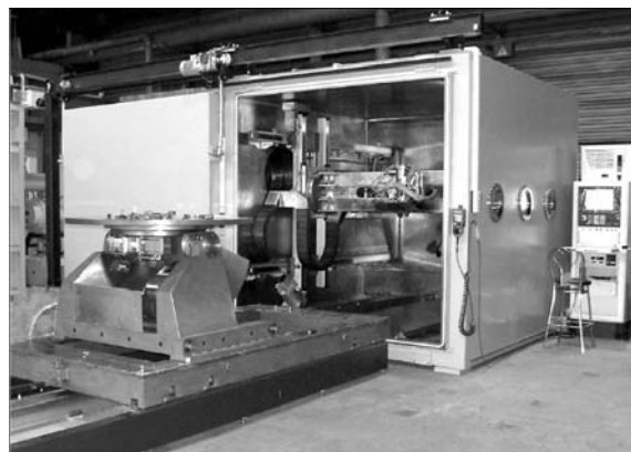
Figure 11. KL-132 machine with seven-coordinate system of welding displacements for making aerospace products
