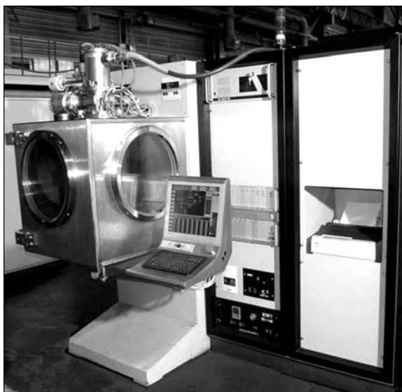
Figure 7. SV-112 machine for welding small-sized items (seven such machines are now operating in industry)
