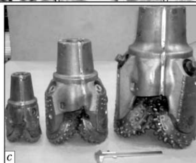
Figure 10. Three-gun machine for welding drill bits (a), butt image (b) obtained in secondary electrons on the display, and general view of welded drill bits of three type-sizes (c) (machines operate at «Volgaburmash» Association, Samara, RF; «Smith Tolls», Ponka City, USA)
