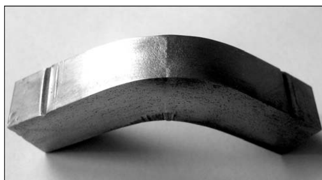
Figure 7. Appearance of the specimen without mechanical notch, cut out from the sound FBW joint, after the test to 3-point impact bending
