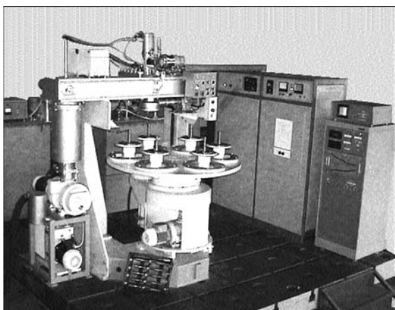
Figure 9. Cycle machine UL-157 for welding gear modules (AVTO-ZAZ Plant, Melitopol, Ukraine))
