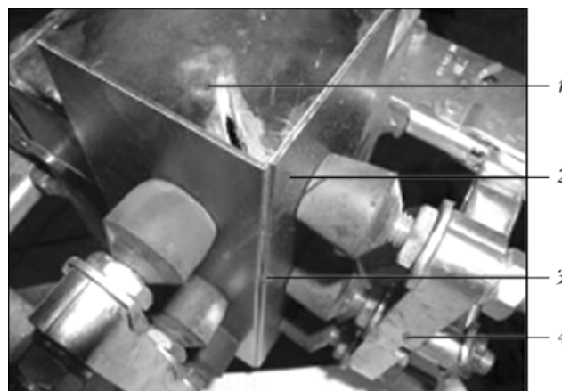
Figure 2. Set-up of metal plate before the welding process: 1 — support for the sheet plates; 2 — sheet plates; 3 — corner joint; 4 — hold-down clamp
