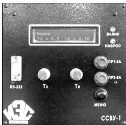
Figure 2. Front panel of communications controller
