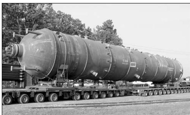
Figure 4. Stainless steel clad hydrotreater reactor (diameter 4500 mm, weight of more than 1000 t)
