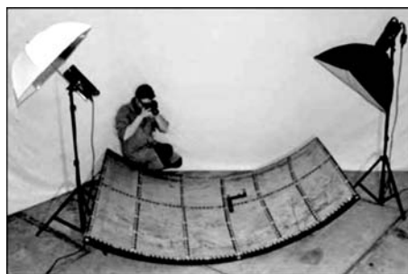
Figure 21. Shape determination of a 60 mm thick explosive formed stainless steel panel with photogrammetry using circular barcodes
