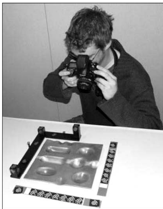
Figure 4. Making digital pictures for photogrammetry analysis
