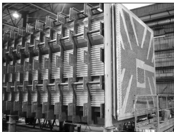
Figure 6. Condenser for electric power generation plant with titanium tubes and titanium clad tubesheets
