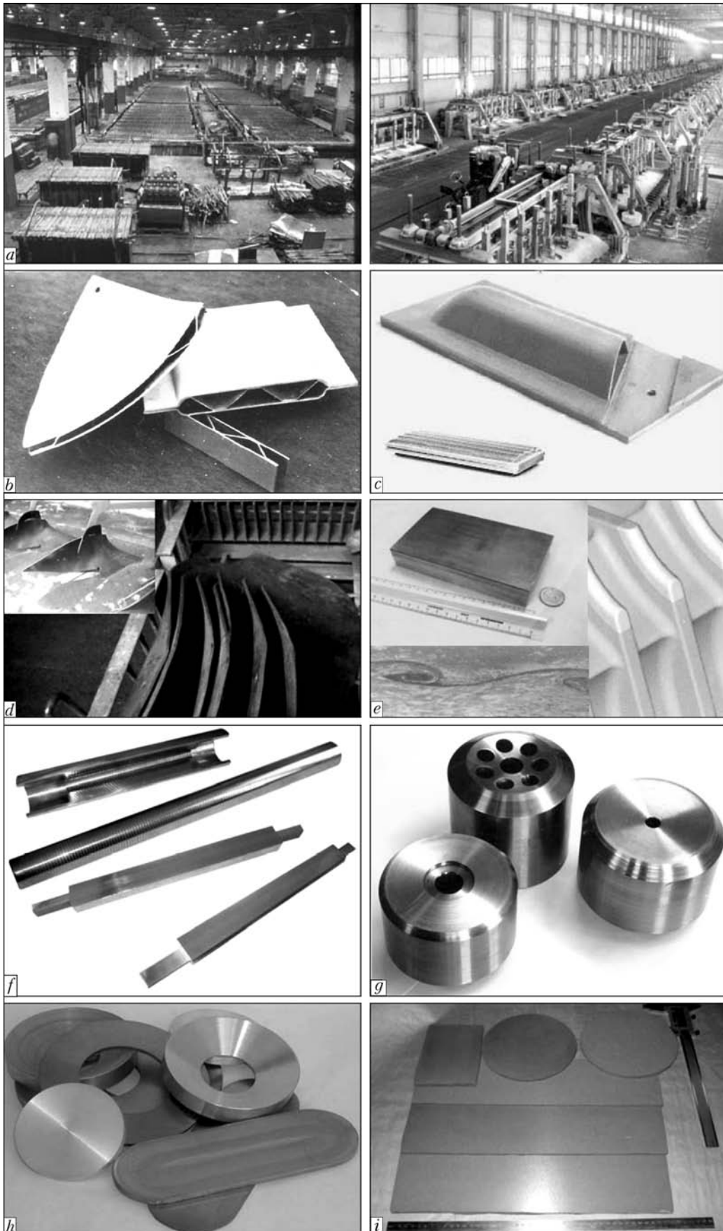
Figure 8. Materials and products made by explosion welding and consolidation: a – copper–titanium and aluminium–steel adapters characterised by increased heat resistance for electrolytic cells; b – panels of light aluminium alloys; c – titanium–copper and aluminium–titanium heat exchangers; d – movable operating elements of tillage machines; e – zirconium bronze and molybdenum billets; f – multilayer composite materials; g – billets for coaxial piston pumps; h, i – composite products for microelectronics – Cr, Ti–W, Ni–Cr–Si ( h ), and silicides Ti, W, Mo, Ta ( i )
