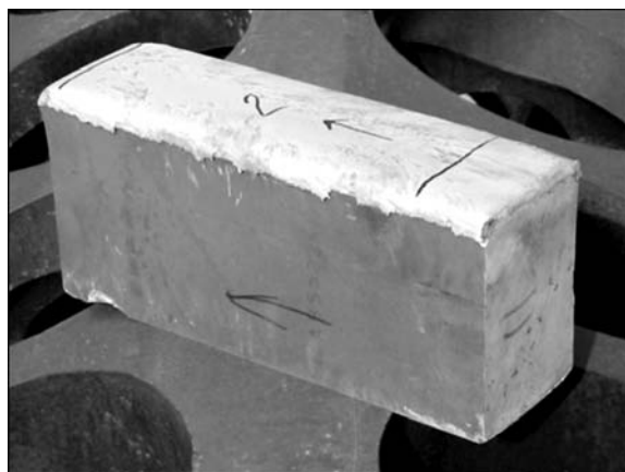
Figure 1. Appearance of a sample after explosion cladding
