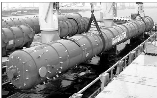
Figure 3. Titanium clad column for PTA manufacture (diameter 5000 mm, weight 450 t)
