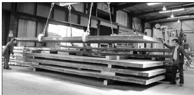
Figure 1. Explosion clad plates to be used for construction of a nickel laterite pressure acid leaching autoclave (plate size of 2200 × × 8000 mm × (10 mm titanium + 117 mm steel))
