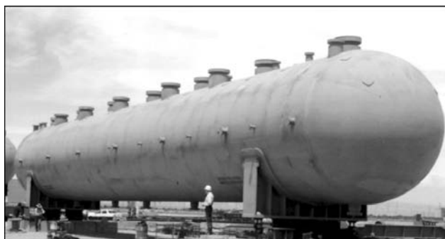
Figure 5. Titanium clad autoclave for pressure acid leaching of nickel and cobalt from laterite ores (diameter 5100 mm, weight 1100 t)
