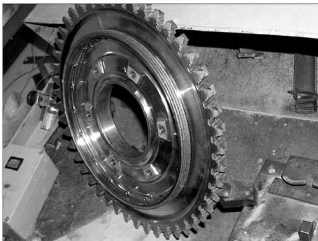
Cladding of labyrinth disk
