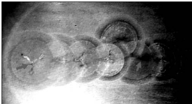
Figure 1. Transverse macrosection of specimen of steel 35L of 500 \times 300 \times 500 mm size with hot cracks formed after ESW of holes of 50 mm diameter and 500 mm depth
