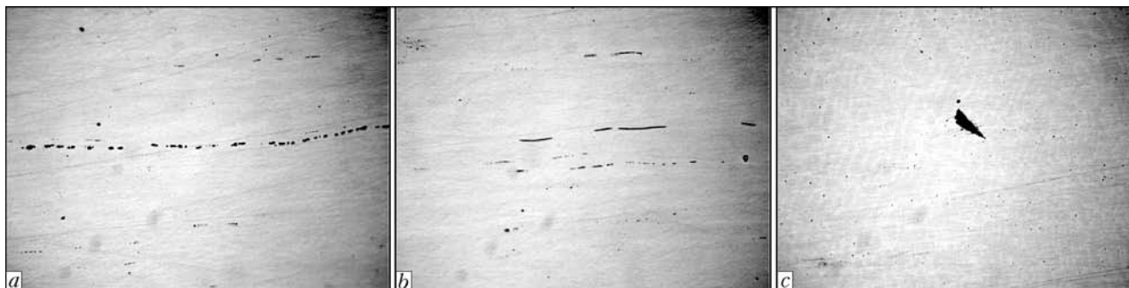
Figure 2. Microstructures ( \times 500 ) of base and weld metal with nonmetallic inclusions in them: a — chains of oxides in BM along the rolling; b — sulphides in BM elongated along the rolling; c — inclusions of corundum and silicates in a single-pass metal
