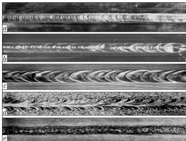
Figure 3. Appearance of welded joints of alloys AMg6 (a), 1201 (b), AMg3 (c), AD0 (d) and IMV-2 (e) made by EBW under the conditions of short-time zero gravity in Tu-104A FL
