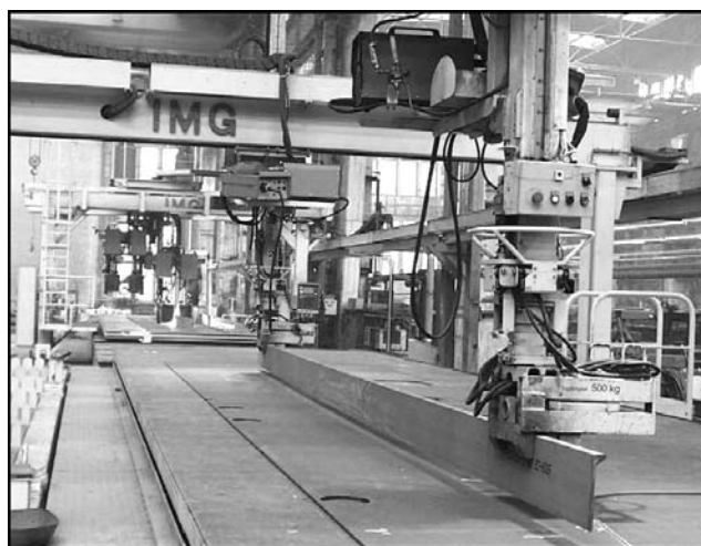
Figure 1. Mounting gantry for stiffeners in micropanel line
