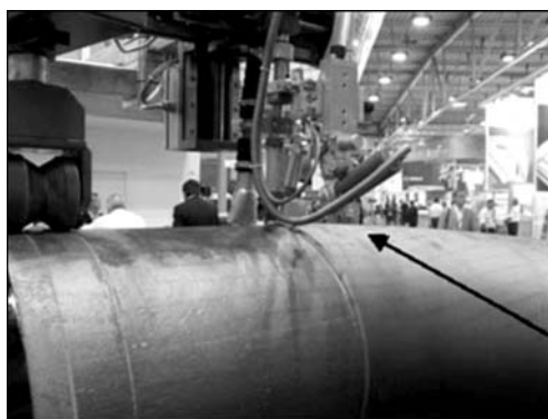
Figure 8. Working body of the following system mounted on the welding head
