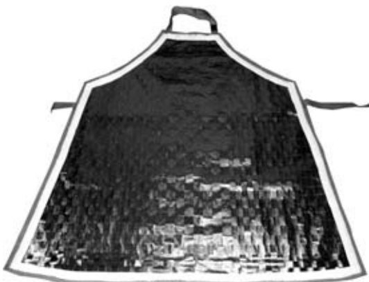
Figure 3. Test sample of welder's protective apron without a lining (reverse side view)
