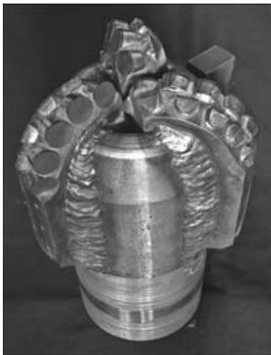
Drill bit and calibrator for extraction of sprayed mining methane
