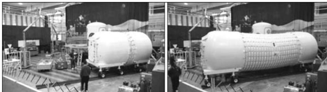
**Figure 10.** Stages of X-Hab module transformation [6]
