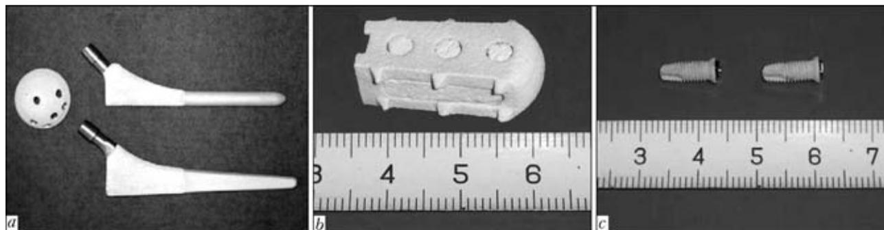
**Figure 4.** Examples of items with bio-cermet coatings produced by microplasma spraying: *a* – hip joint endoprosthesis; *b* – cermet implant for interbody vertebral spondylosyndesis; *c* – dental implant
