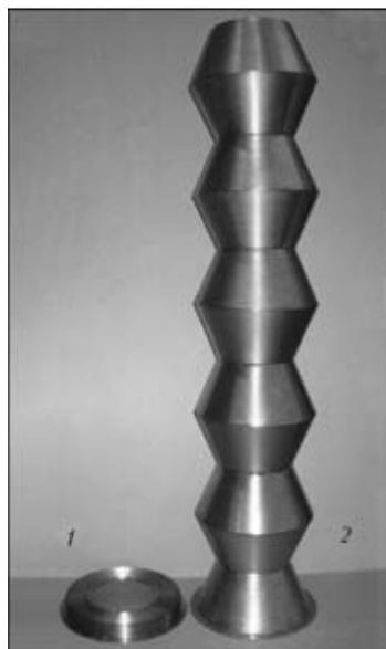
**Figure 2.** TS of a periodic profile (material – VT1-0 titanium 0.15 mm thick), consisting of 11 basic conical shells [2]: 1 – structure in the compact folded state; 2 – deployed structure
