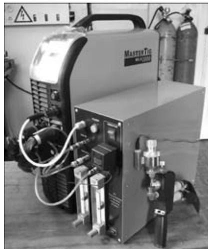
Figure 1. Appearance of microplasma spraying system MPN-004
