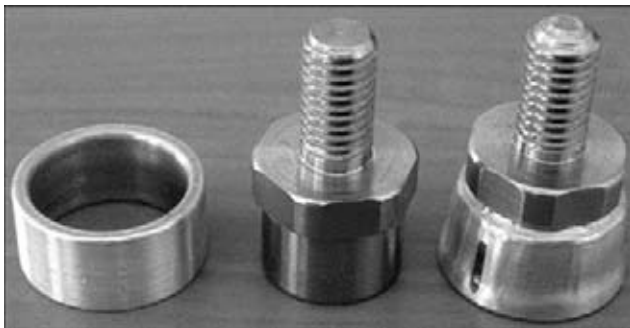
Figure 8. Aluminum ring MP-welded to steel bolt
