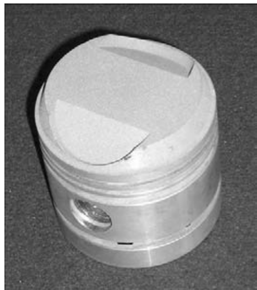
Figure 7. Piston of aluminium alloy with thermal barrier coating
