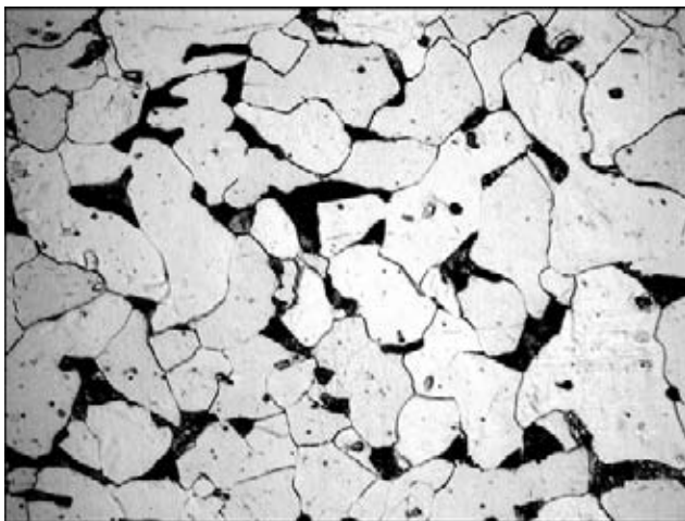
Figure 1. Microstructure (x500) of steel VSt3sp
