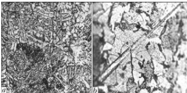
Figure 3. Fatigue changes of microstructure of HAZ metal of 09G2S steel butt welded joints: a – N = 230,000 cycles, \sigma_a = 120 MPa; b – N = 720,000 cycles, \sigma_a = 80 MPa ( a – \times 500 ; b – \times 1000 )
