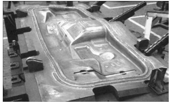
Figure 5. Die block of GAZ car after plasma hardening of pressure loop
