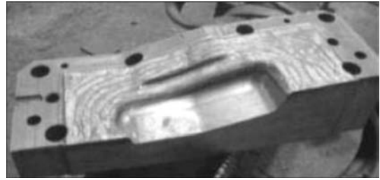
Figure 4. Fragment of split die after plasma hardening
