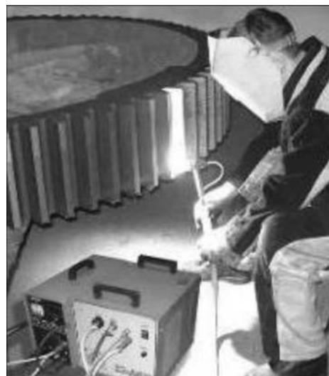
Figure 7. Plasma hardening of teeth of coarse-pitch gear
