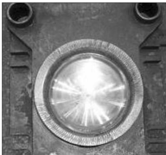
Figure 1. Die block for cutting of receiver bottoms after plasma hardening
