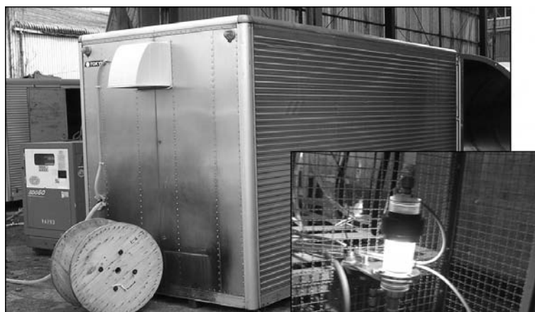
General view of mobile plasma unit for treatment of radioactive water
