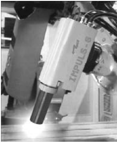
Figure 1. Pulse plasmatron for surface hardening treatment
