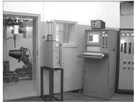
Figure 3. General view of the unit for pulse plasma hardening treatment of surfaces of parts, including for thermal spraying of coatings
