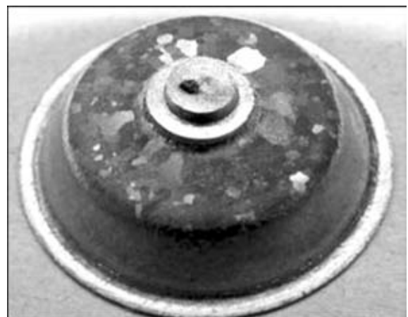
Figure 6. Shifting of ion crater relative to cathode center
