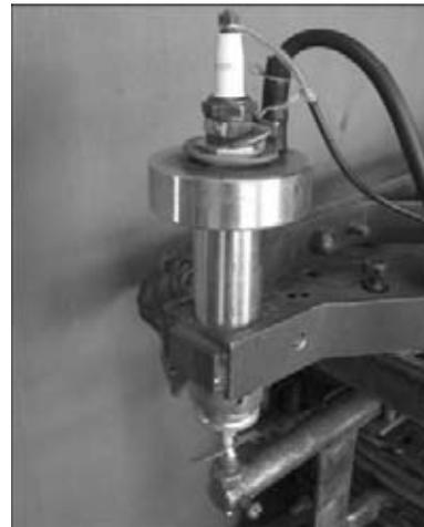
**Figure 3.** Welding head with explosion type mechanism of impact treatment of the weld
