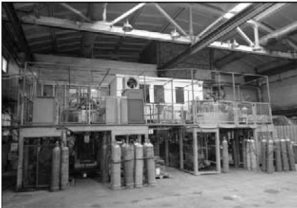
Unit for thermal centrifugal spraying SFERA-2500
