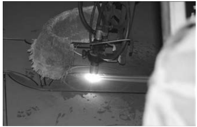
Figure 4. Process of cutting (plasma-forming medium – air + water)
