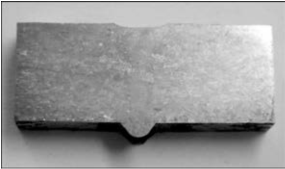
Figure 4. Macrosection of welded joint of alloy 1 made by EBW with 200 °C preheating
