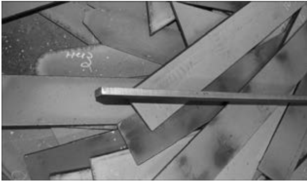
Figure 8. Appearance of billets after plasma cutting
