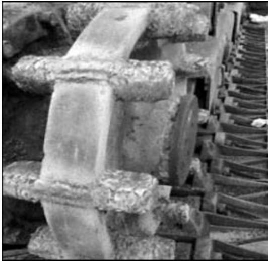
Figure 4. Appearance of repaired drive sprocket of crane KS8165
