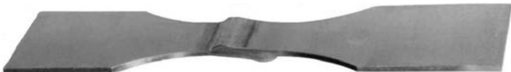
**Figure 3.** Sample of overlap joint for fatigue testing
