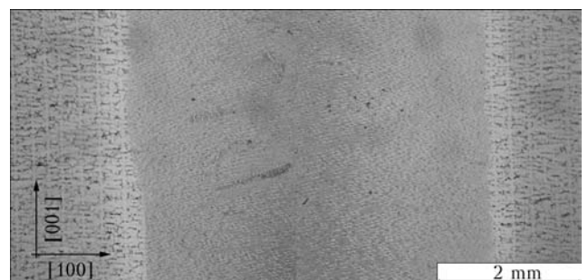
Figure 1. Microstructure of weld metal of JS26 alloy welded joint with symmetrical crystallographic orientation
