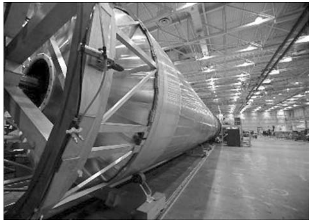
Figure 6. Tank of rocket-carrier «Falcon 9» of Al-Li alloy (SPACEX), the longitudinal and circumferential welds of which are produced using FSW. Formation of hydrogen bubbles is completely eliminated (access mode: http://en.wikipedia.org/wiki/File:SpaceX_factoryFalcon_9_booster_tank.jpg )
