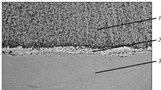
**Figure 3.** Microstructure ( $\times 300$ ) of brazed DHC + steel joint before drill bit testing: 1 – hard alloy VK8; 2 – brazed seam; 3 – steel 30Kh
