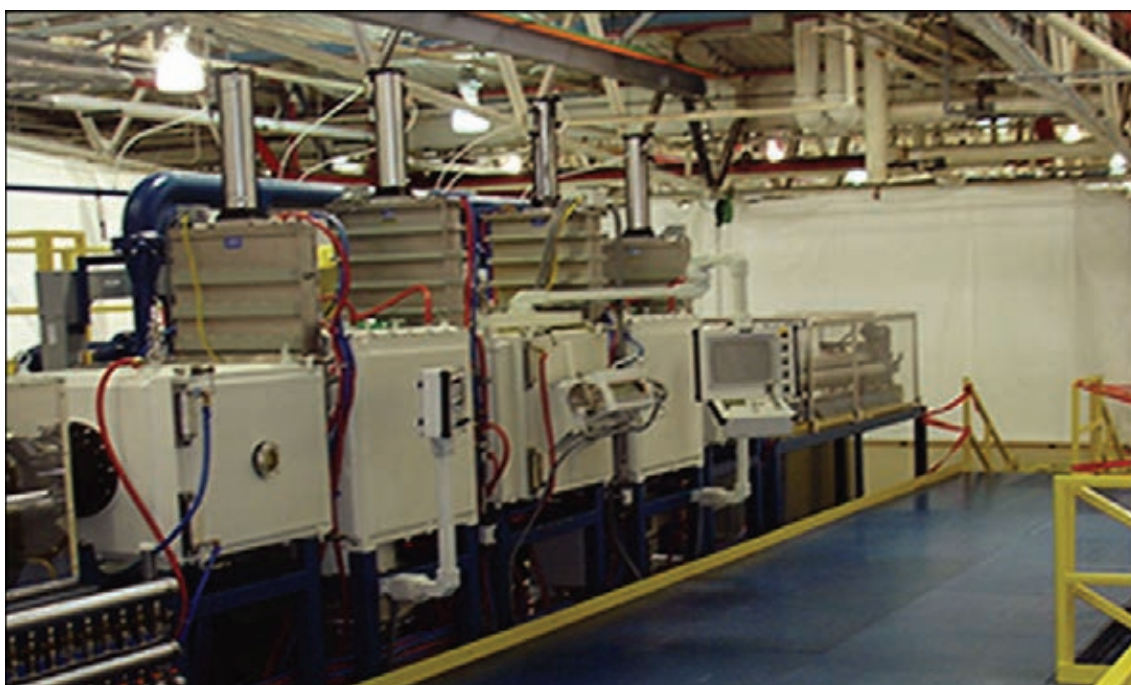
Designed and manufactured at Pratt&Whitney-Paton EB unit for deposition of protective coatings on aircraft gas turbine blades at customer facility
