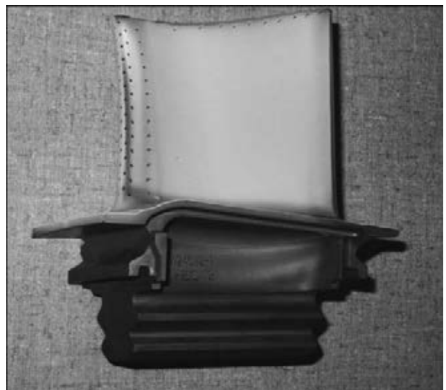
Commercial gas turbine blade with thermal barrier coating
