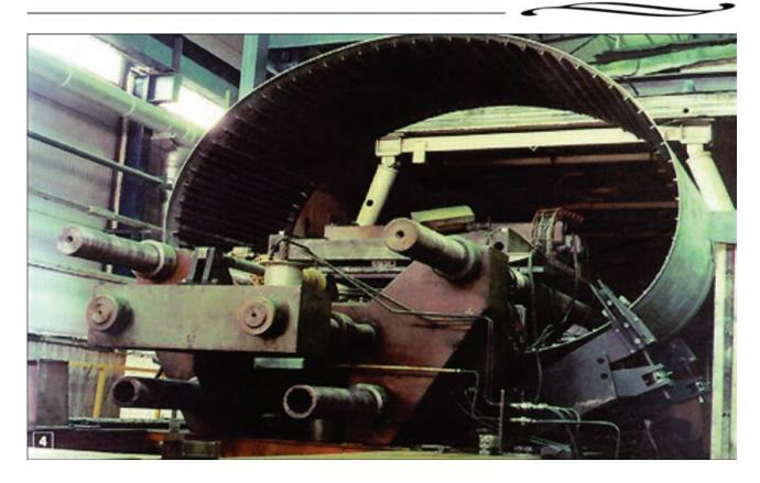
assembly-welding units that combine distorting systems, equipment for mechanical treatment of welded edges under the conditions of preset loading and specialized welding equipment.
