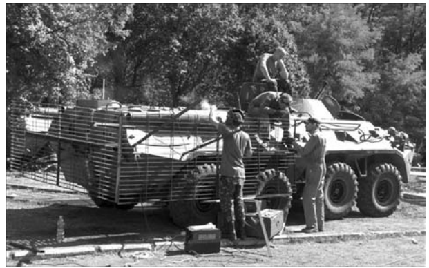
Assembly of anti-cumulative screens on armored personnel carrier BTR-80 of the Armed Forces of Ukraine in the ATO zone by the Chair staff members
