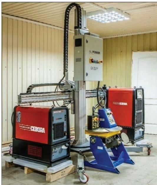
Innovative universal equipment for plasma, hybrid and combined (tandem) plasma-MIG welding, developed at PWI and delivered to the laboratory and technological base of CUWI in Guangzhou
