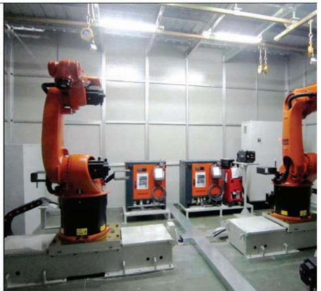
Laser welding and cutting as well as hybrid laser welding with two robots using 10 kW laser at the laboratory and technological base of CUWI in Guangzhou (deep penetration laser welding, hybrid laser-MIG welding, laser welding using scanning, laser welding using two beams, 3D laser cutting)
