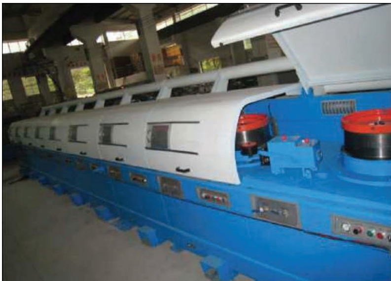
Line for production of flux-cored wires for arc welding, surfacing and thermal spraying at the laboratory and technological base of CUWI in Guangzhou
