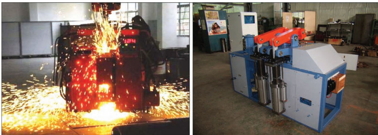
Equipment for flash-butt welding, developed at PWI and delivered to the laboratory and technological base of CUWI in Guangzhou
