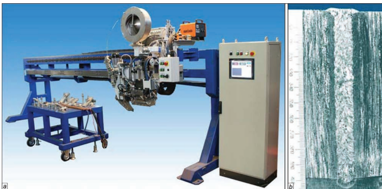
Prototype of machine for producing welded joints of titanium and titanium alloys of up to 4 m length and up to 120 mm thickness (a), and macrosection of welded joint of titanium of increased thickness (b)
