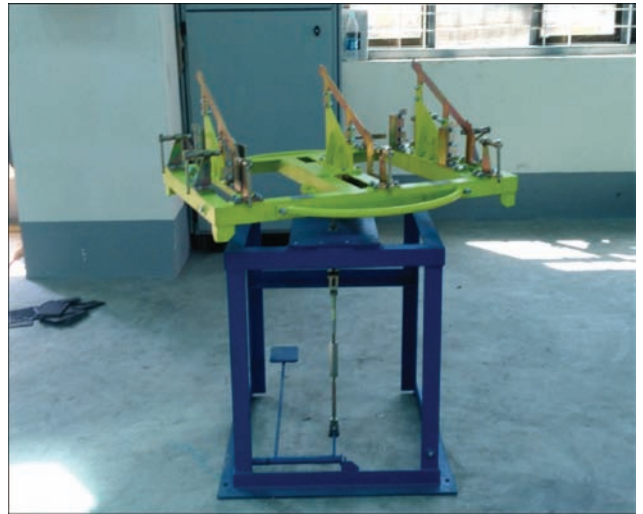
Installation for assembly and welding of motor compartment elements
