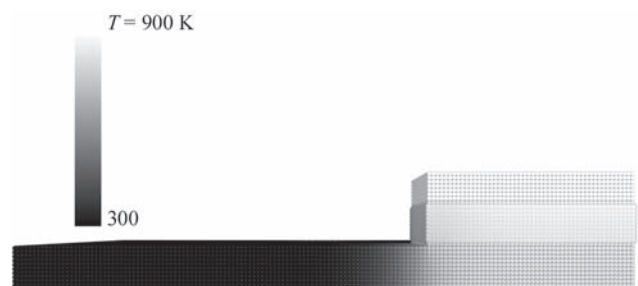
Figure 7. Distribution of temperature in cross-section of system (1/4 of its part is shown) at its local heating in the moment of solder melting. Length and width of second plate 3 times exceed length and width of first plate
