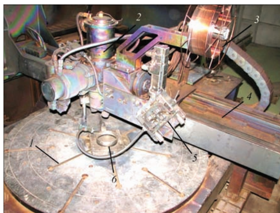
Figure 6. Location of equipment for surfacing with wire in vacuum chamber (description 1–6 see in the text)
