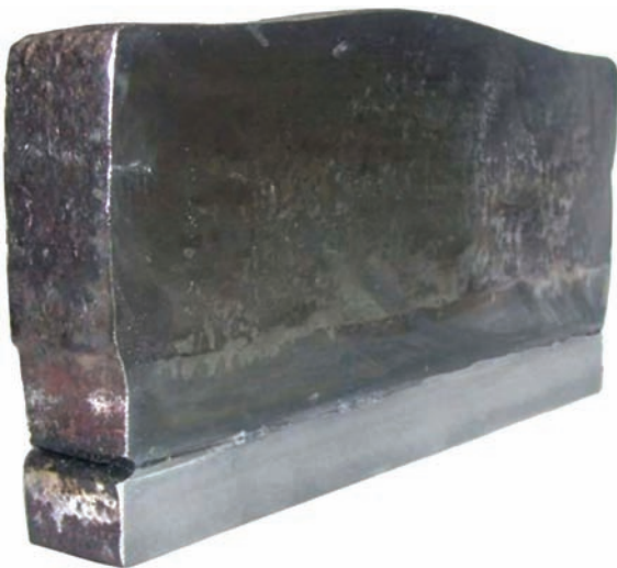
Figure 4. Appearance of side surface of the deposited layer with application of AN-26 flux at initial value of L_0 equal to 70 mm (longitudinal section of the deposited billet)
