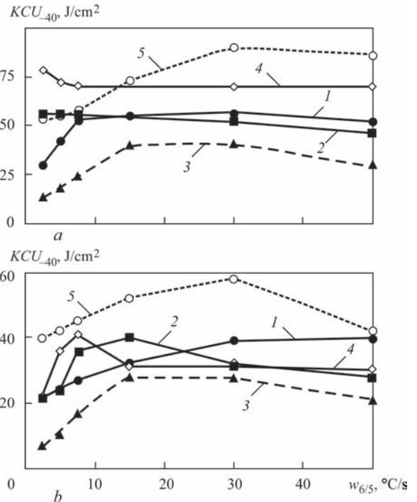
**Figure 2.** Influence of cooling rate  $w_{6/5}$  on  $KCU_{-40}$  (a) and  $KCU_{-40}$  (b) of metal in the region of overheating of HAZ of steels: 12GN2MFAYu (1), 14Kh2GMR (2), 14KhG2SAFD (3), 14KhGN2MDAFB (4), 12GN3MFAYuDR-Sh (5)
