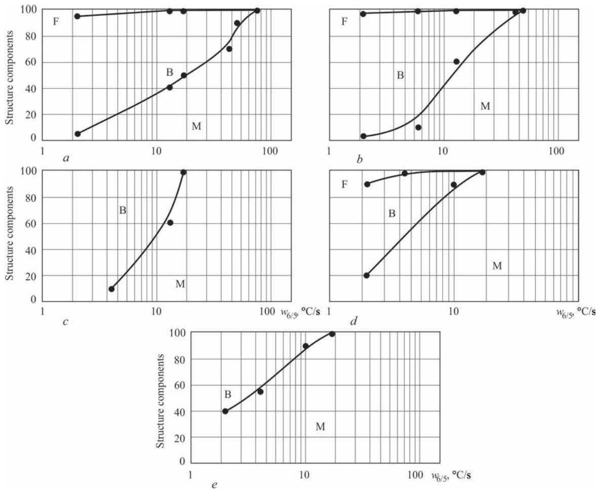
**Figure 1.** Diagrams of structural transformations of austenite in the overheating region of HAZ metal of high-strength alloyed steels 12GN2MFAYu (a), 14KhG2SAFD (b), 14Kh2GMR (c), 12GN3MFAYuDR (d) and 14KhGN2MDAFB (e)
