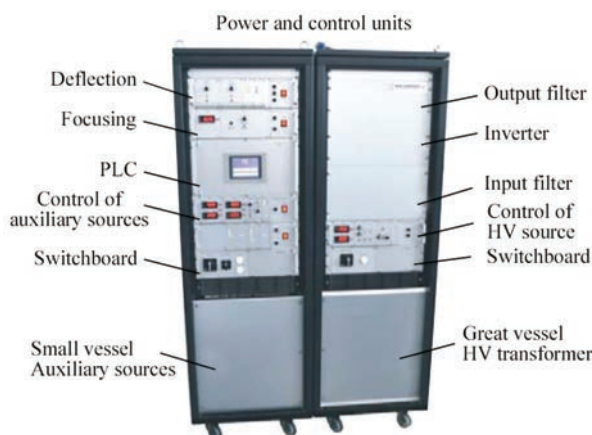
Figure 1. The powerblock type PZ EB 30
