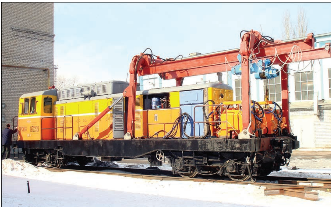
Mobile rail welding complex on railway platform
