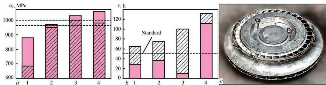
**Figure 11.** Tensile strength of butt brazed joints (a) produced using filler metals of the system: Ni–Pd–Cr–Si (1); Ni–Pd–Cr–Co–Si (2); Ni–Pd–Cr–B (3); Ni–Pd–Cr–Ge (4); long-term strength (b); double shrouded centrifugal wheel of axial flow compressor of gas-turbine engine (c)
