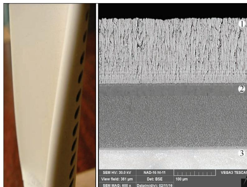
Appearance and microstructure of gradient thermal barrier NiCoCrAlY(AlCr)/ $\text{ZrO}_2$ –8 %  $\text{Y}_2\text{O}_3$  coating on a blade of gas turbine engine:
