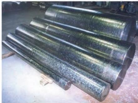
Titanium ingots of 100–600 mm diameter
