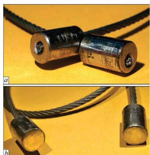
**Figure 14.** Braze elements of high-strength austenitic steel and steel 45 before (a) and after brazing (b)
