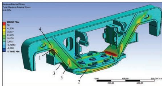
**Figure 2.** Distribution of main stresses in the structure of welded side frame under the action of loads regulated by the Standards [6] (description 1–5 see in Table 2)
