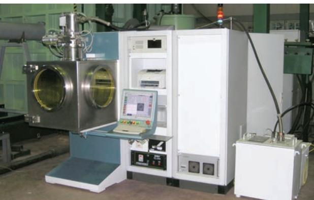
Small-sized electron beam installation
