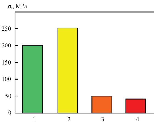
**Figure 6.** Strength of brazed Cu–W joints: in the initial state after brazing (1); after neutron irradiation in the SM-2 reactor at  $T = 100^\circ\text{C}$  and a dose of  $5\text{--}10^{21}\text{ neutron/cm}^2$  (2); at  $T = 310^\circ\text{C}$ , in the SM-2 reactor, dose of  $5\text{--}10^{21}\text{ neutron/cm}^2$  (3); in the BOR-60 reactor at  $T = 400^\circ\text{C}$ , dose of  $5\text{--}10^{22}\text{ neutrons/cm}^2$  (4)
