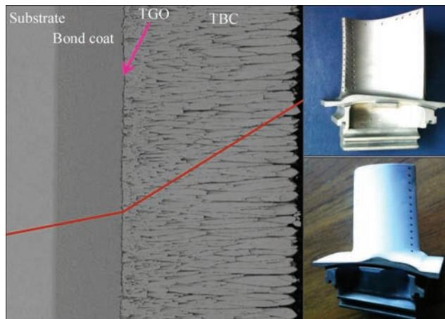
**Figure 2.** Thermal barrier coating and appearance of blades with metal and ceramic coatings
