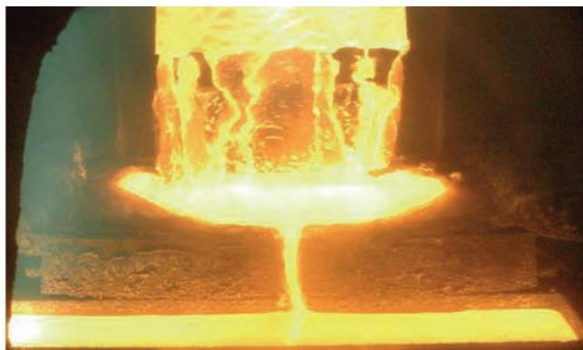
Producing 165×950×2500 mm slab-ingot of PT-3V titanium alloy
