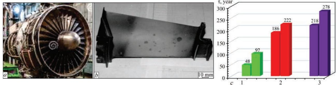
**Figure 12.** Gas-turbine engine (a), blade (b), long-term strength of butt similar brazed joints Ni<sub>3</sub>Al+Ni<sub>3</sub>Al produced using multicomponent nickel brazing filler metal without heat treatment (1), with heat treatment (2) and dissimilar joints Ni<sub>3</sub>Al+ZhS6U with heat treatment
