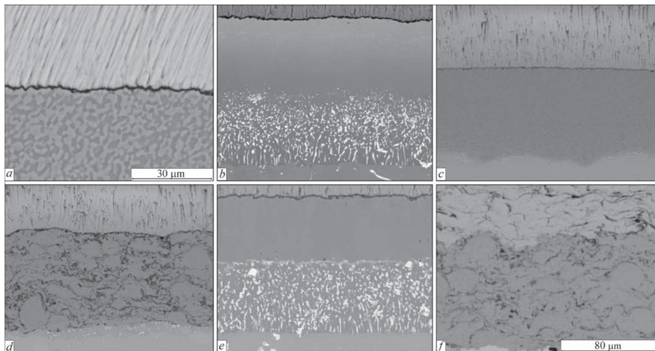
**Figure 3.** Different types of bond coats in thermal barrier systems of coatings produced by EB-PVD: (a–e) and APS: a — EB-PVD; b — PtAl; c — LPPS; e, f — HVOF; e — NiAl
