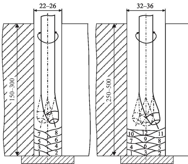
**Figure 2.** Examples of bead arrangement by the optimized technology of narrow-gap welding
