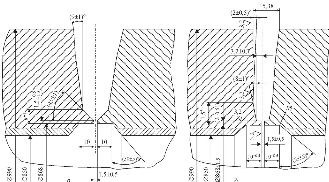
**Figure 8.** Edge preparation: *a* — standard; *b* — proposed
