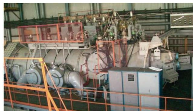
All-purpose electron beam installation UE5810
