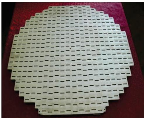
Figure 1. General view of brazed antenna array
