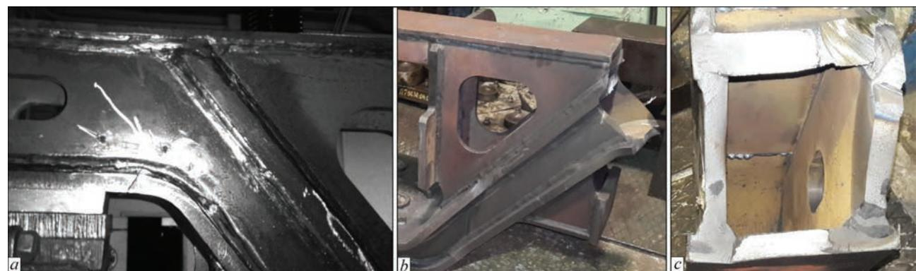
**Figure 6.** Fragment of fracture of test specimen No.2 of all-welded side frame after macrocrack formation during accelerated fatigue tests (a) and after fracture in the radius blend zone R55 of axial hole (b, c)
