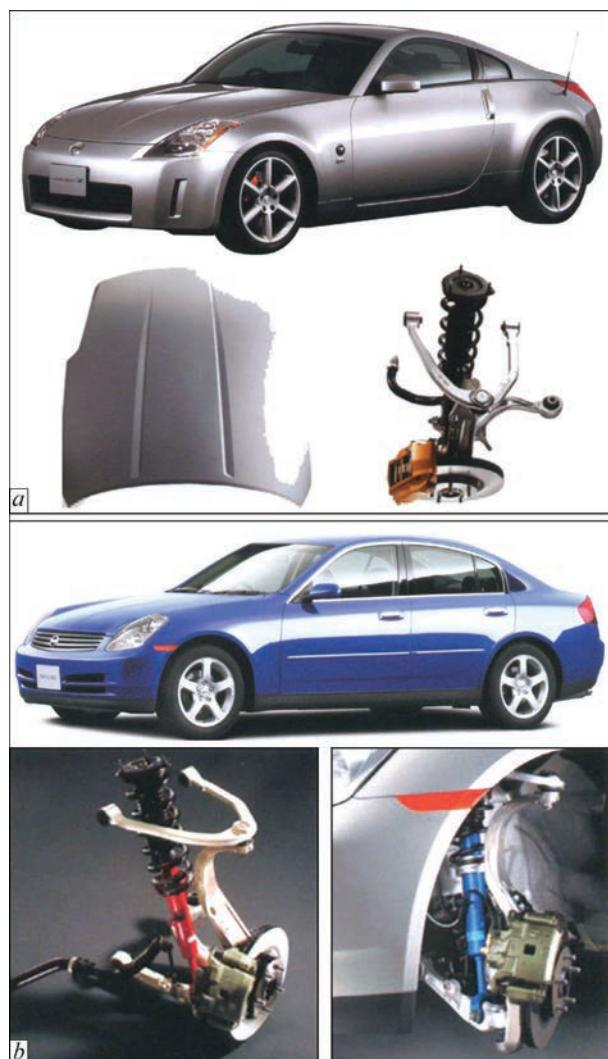
**Figure 5.** Examples of aluminium alloy application in passenger cars: a — Feardi Z33; b — Skyline V35
