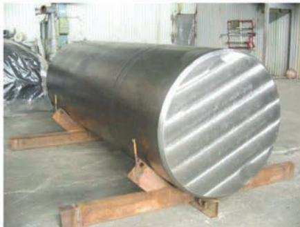
Titanium ingot of 1100 mm diameter
