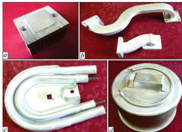
Figure 3. Brazed products of aluminium alloys: a — plate aluminium heat exchanger; b — element of ultra-high frequency module; c — tubulat heating elements for household appliances (d)
