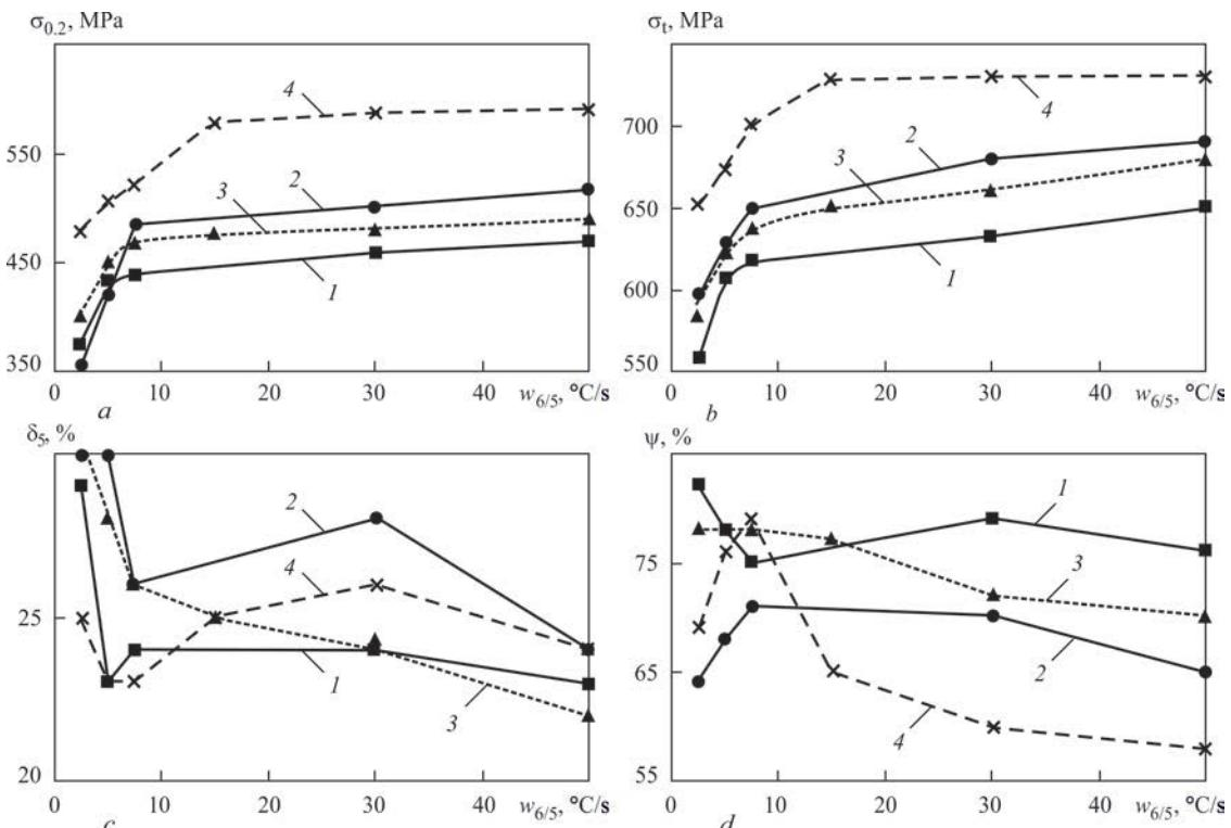
Figure 2. Effect of cooling rate  $w_{6/5}$  on the values of yield strength (a), tensile strength (b), elongation (c) and reduction in area (d) of HAZ metal of steels: 06GBD (1); 09G2SYuch (2); 06G2B (3); 10G2FB (4)
