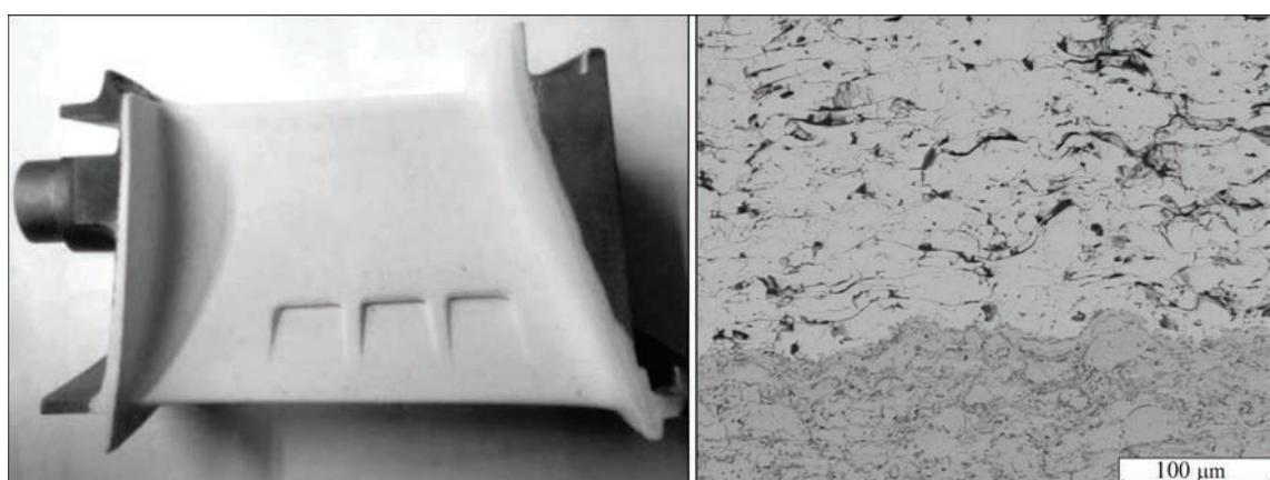
**Figure 5.** Blade with thermal barrier coating, produced by the methods of HVOF/APS and structure of the interphase between the metal (HVOF) and ceramic (APS) layers of TBC system
