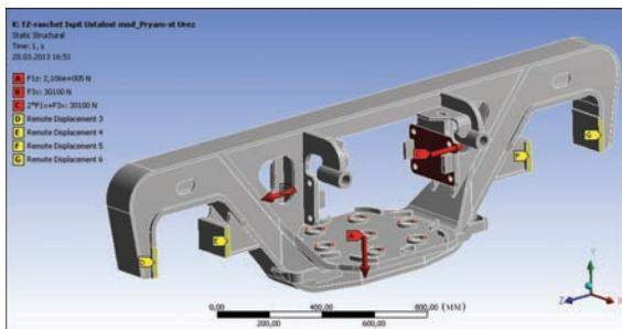
**Figure 1.** Vertical load  $F_{lz} = 210.6$  kN (A), uniformly distributed over the area of spring suspension on the support surface of the central spring suspension, and the wedge span force  $F_{3x} = 30.1$  kN (B), which are applied to the vertical posts of the central spring hole
