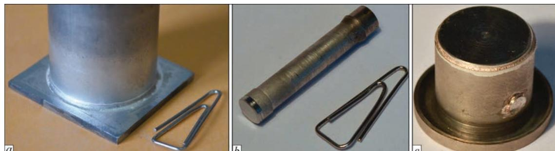
**Figure 8.** Brazed specimens of dissimilar materials kovar–titanium alloy: model specimen for tests on sealing (a); tubular element (b); brazed assembly with plug (c)
