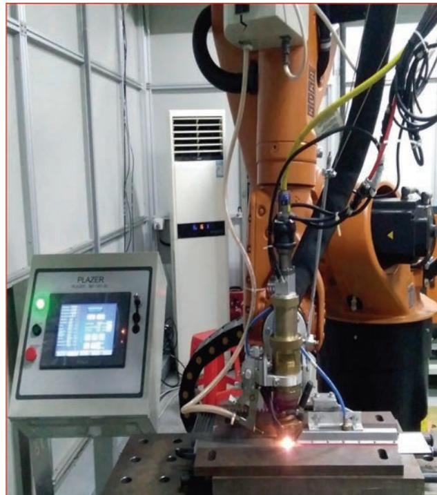
Robotic technological complex for high-speed hybrid laser-plasma welding
